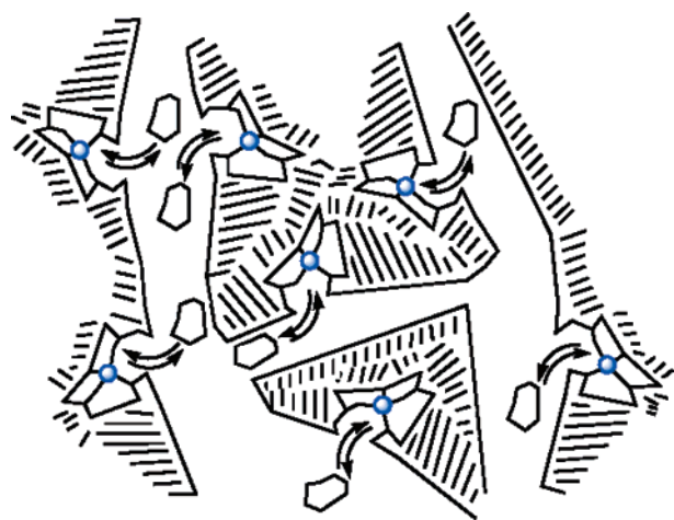
FIGURE 1. Schematic illustrating a porous solid containing immobilized metal complexes. Blue spheres represent the metal ions, and the hash lines symbolize the porous amorphous host.
